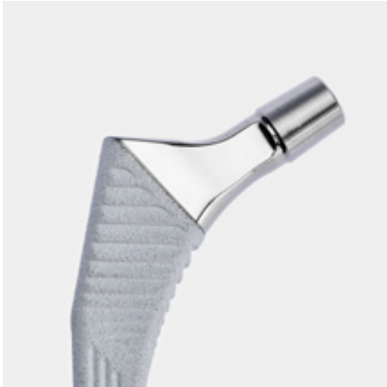
Expe rsus Hip Stem STD 135°, Ti6Al4 V, ISO 5832-3, TPS- and HA-coating
